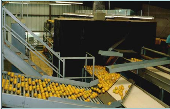
Enclosure Within Which Fruits are Sorted Under UV Light to Eliminate Defects
